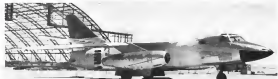
NEW JATO BOTTLES are being tested on the RB-66 at Edwards AFB. Steps toward tail behind JATO installation on transition sensitive front components, ends with a different seating gear. When tests on tail temperatures at various locations are determined by the actual pilot, New JATO bottles were required because of the old configuration, were showing the loading when dropped. Bottles mounted there are made by Phillips Petroleum Products. Other units used on four Ansony General and A1G when Robinson Laboratories
